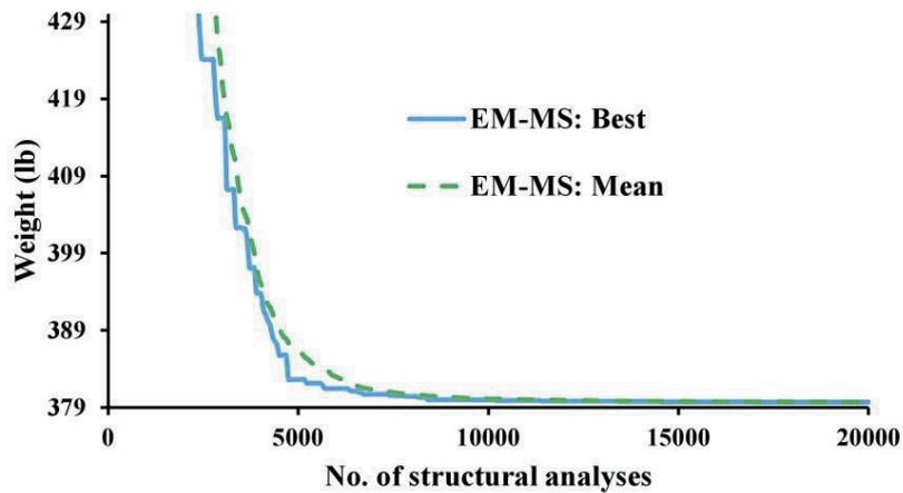
Fig. 9 The convergence diagrams of the EM-MS algorithm for the 72-bar spatial truss structure.
