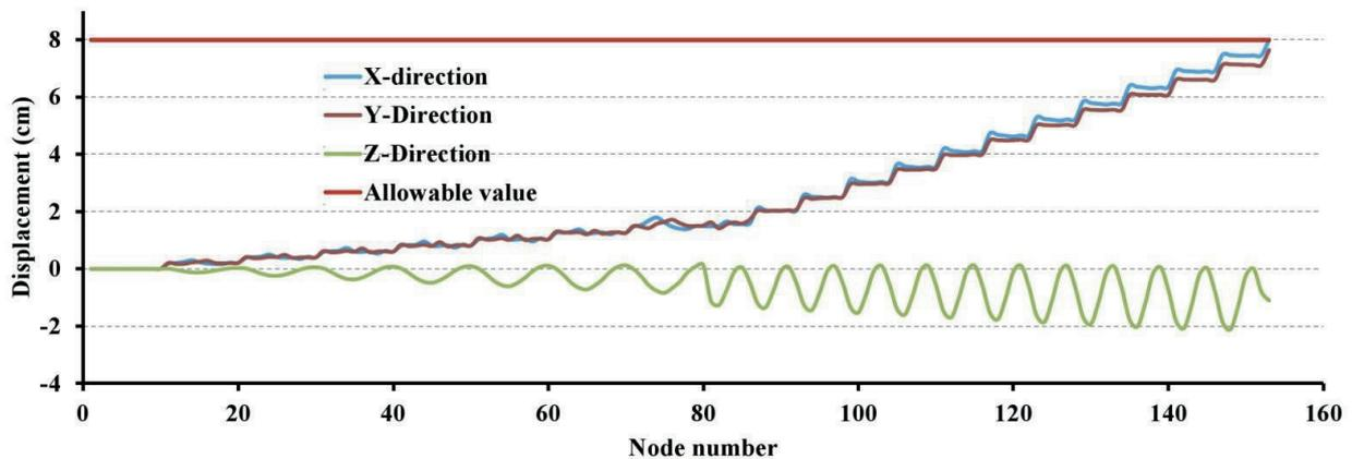
**Fig. 11** Comparison of existing and allowable displacements in X, Y and Z directions in the 582-bar tower truss structure.
