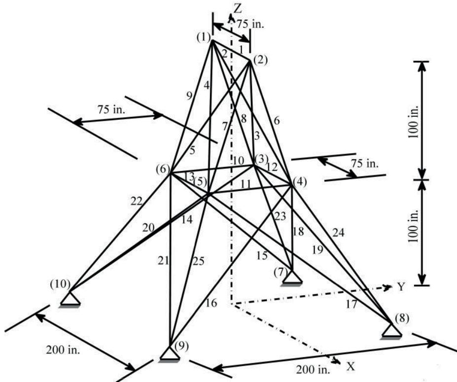
Fig. 6 Schematic of the 25-bar spatial truss structure.
