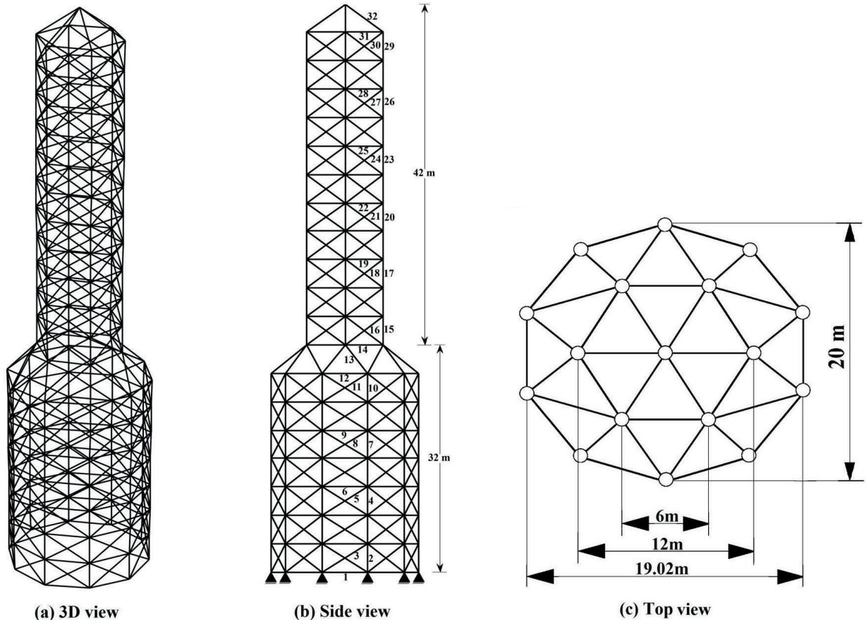
**Fig. 10** Schematic of the 582-bar tower truss structure: 3D, Side and top views.
