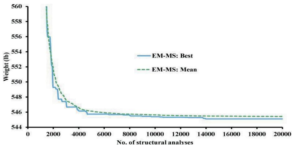
Fig. 7 The convergence diagrams of the EM-MS algorithm for the 25-bar spatial truss structure.
