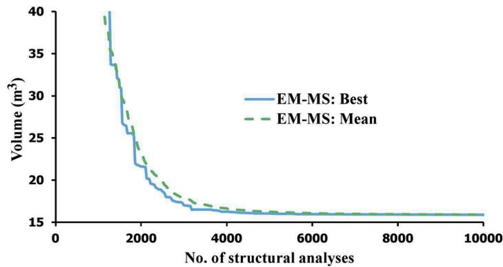
Fig. 13 The convergence diagrams of the EM-MS algorithm for the 582-bar tower truss structure.
