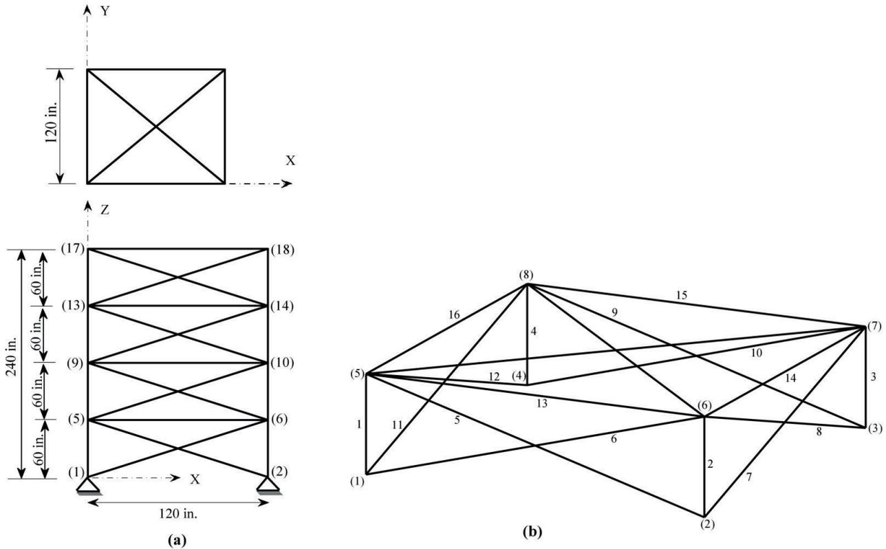
Fig. 8 Schematic of the 72-bar spatial truss structure: (a) Top and side view (b) Element and nodal numbering patterns for first story.
