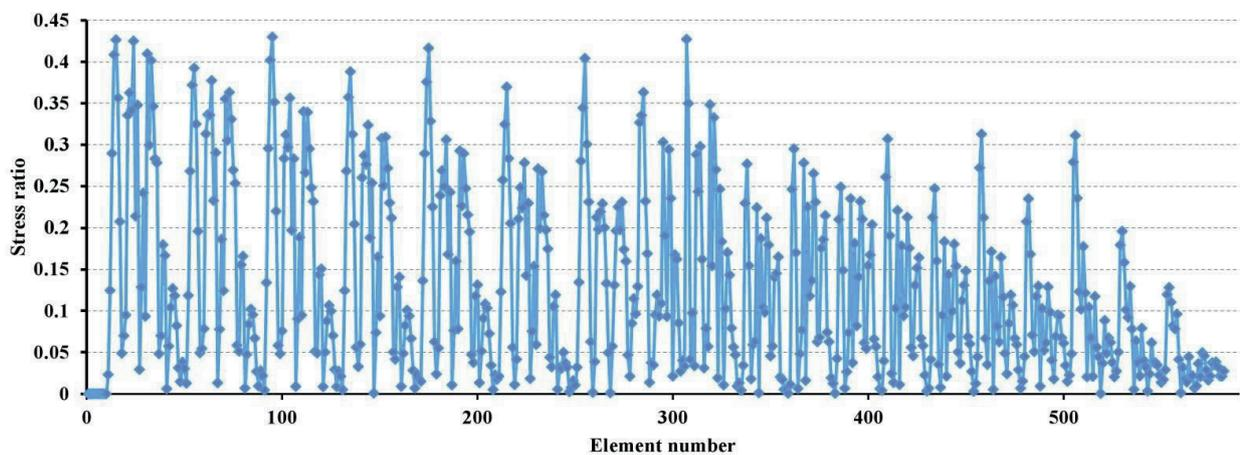
**Fig. 12** The stress ratio of members in 582-bar tower truss structure.
