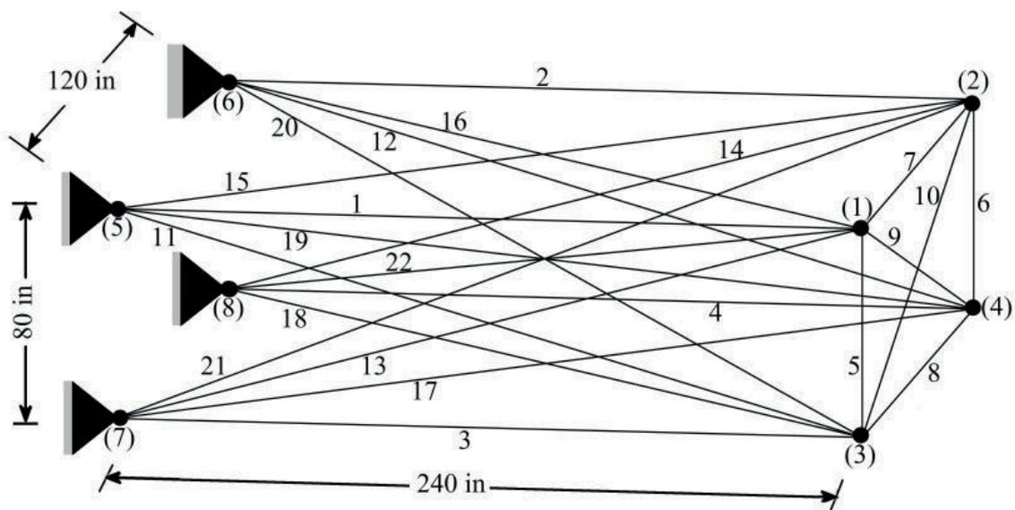
Fig. 4 Schematic of the 22-bar spatial truss structure
