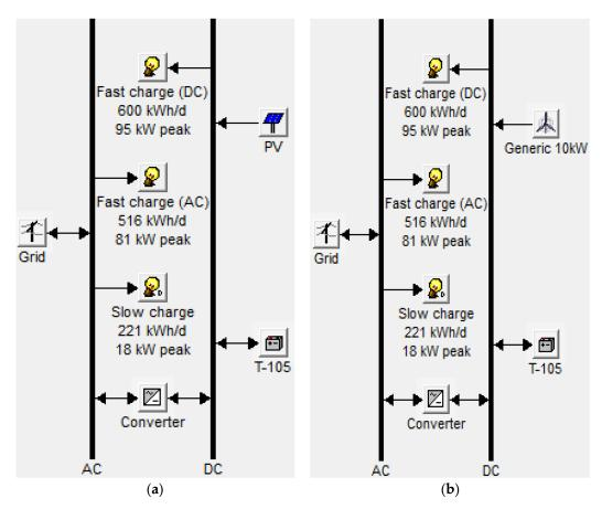
**Figure 5.** Schematic of systems under study in HOMER (a) (Solar-based system (b)) Wind-based system.
