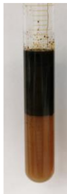
Fig. 13. Emulsion behaviour of 0.8 % Coco Glucoside/Crude Oil with 9.5 g/dL KCl brine.
