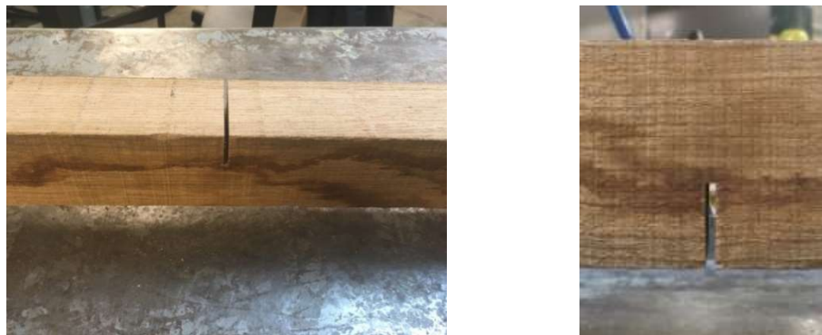
Figure 3. Damaged beam specimens (cut dimensions: 20 x 67 mm).
