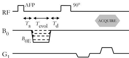
Figure 1: 1D  $T_1$  dispersion pulse sequence
