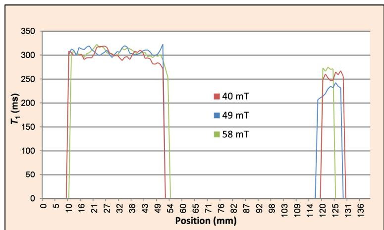
Figure 2: 1D  $T_1$  dispersion profile for an array of  $\text{CuSO}_4$  (left) and albumen (right)
